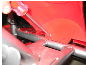
D、 fix the front pane on the frame and fix it with crew 4*10
