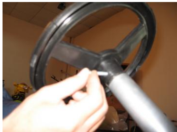
C、 fix the steering wheel on the steering shaft and fix it with screw 5*35
