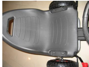
F、 Fix seats with 5*40 screws
