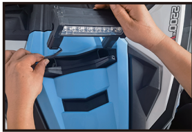
14. Install detective lights
