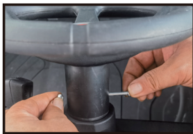
11. Fix the steering wheel
