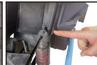
6. Fix the shock absorber
