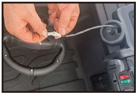
10. Connect the steering wheel
