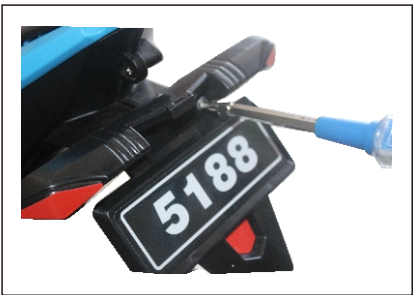
Align the rear card with the rear hole Screwed
