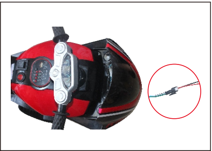
The front of the car is aligned with the front part of the car and pushed forward Just tighten, then turn the front line and the body line connection;
