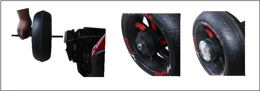
Pass the rear axle into the rear of the body, screw it tightly, and finally fasten the wheel cover (two wheels The installation method is the same)
