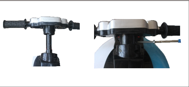
The handlebar is aligned with the body and screwed tightly;
