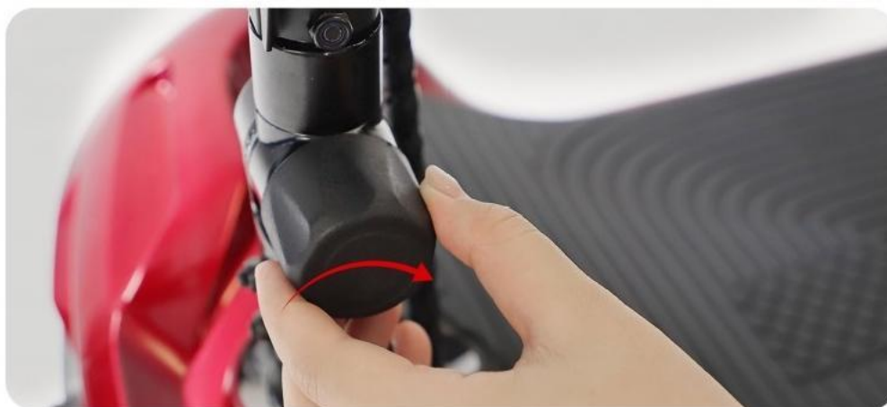
Fig 4. Loosen the tiller adjustment knob
