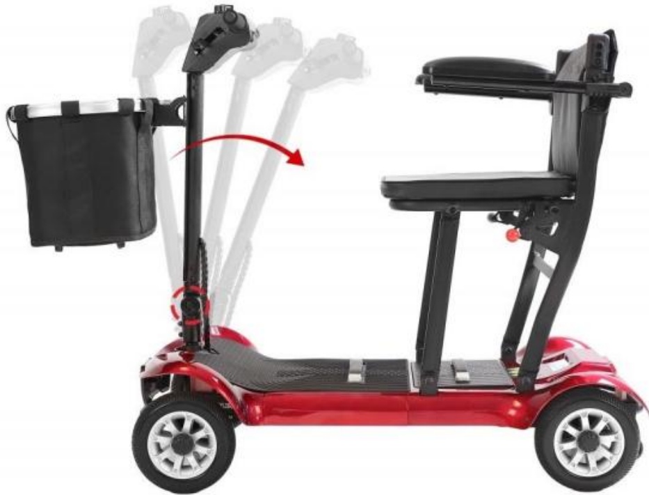
Fig 5. Adjust a proper tiller angle to fit the driver.
