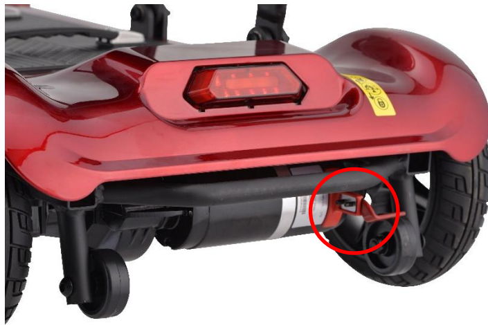
Fig 8. Manually and automatically switch the brake control lever
