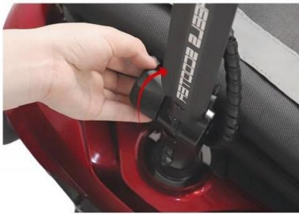
Fig 12 Steps of adjusting the tiller
