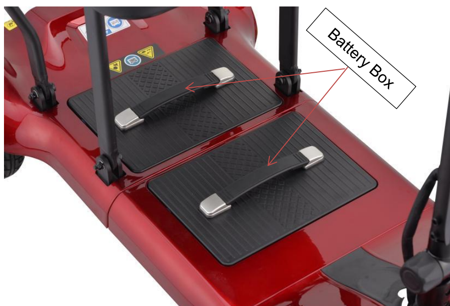
Fig 9 Overview of battery box position
