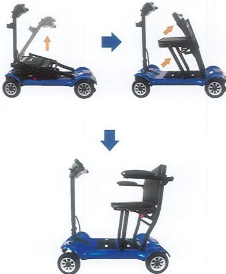
Fig 13 Steps of installing the scooter
