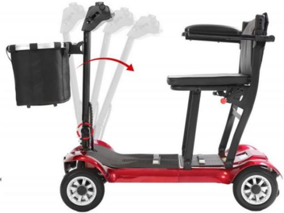
Fig 12 Steps of adjusting the tiller
