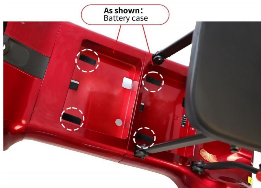
Fig 10 Overview of four fasteners
