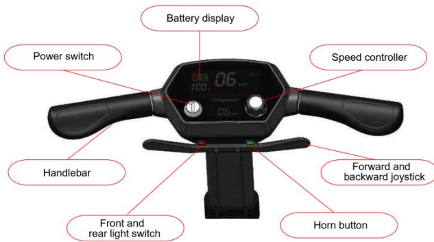
Fig 2. Overview of control console
