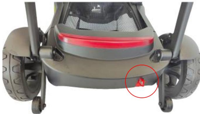
Fig 7. Manually and automatically switch the brake control lever
