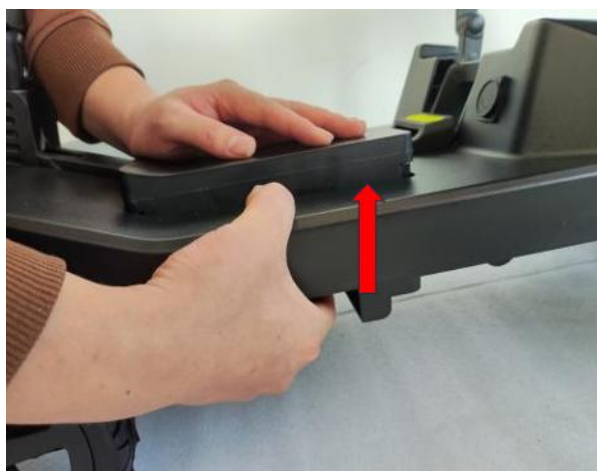
Fig 9. Battery box removal
