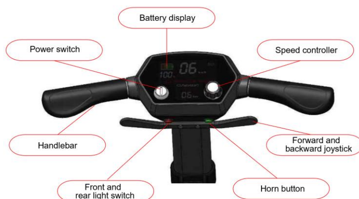
Fig 2. Overview of control console
